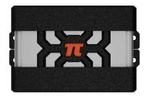
The PI connects to the MnUC via USB cable for Data, Audio and power. The PI (Platform Interface) acts as an Audio Bridge to the MoP for Audio Output and configuration
